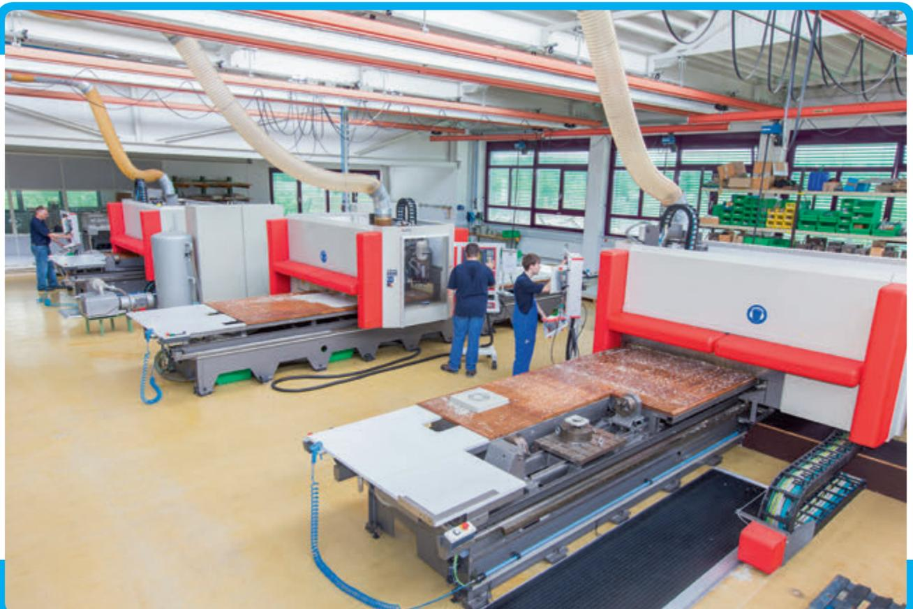
Latest plastics processing on computer-controlled machining centers.
