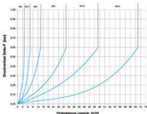
Pressure loss diagram for determining the appropriate filter chamber
