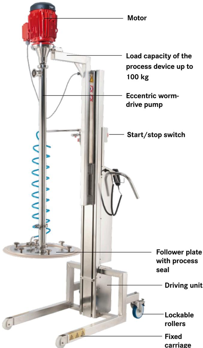
VISCOFLUX mobile, the drum emptying system.
