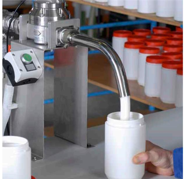
VISCOFLUX mobile – continuous transport using the example of vaseline.
