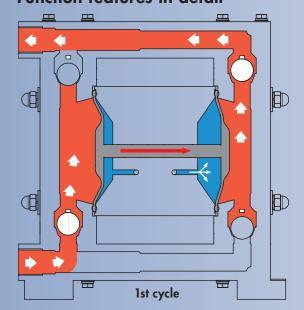
FLUX air-operated diaphragm pumps are positive displacement pumps consisting of two pump housings and one control valve part. Diaphragms within the pump housings securely separate the liquid section (red) from the air section (blue). Both diaphragms are connected by a selector shaft which is located in the control valve part.
