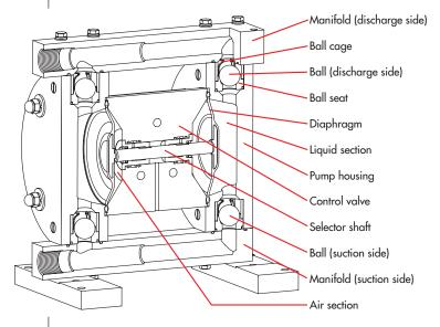
FLUX air-operated diaphragm pumps are most versatile and can be used for almost every liquid in all different fields of industry.
