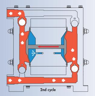
Compressed air inflating alternately the air sections causes a movement of the diaphragms (1st and 2nd cycle). The subsequent transfer operation is controlled by a control valve which is easy to dismantle.
